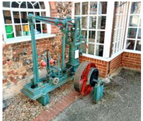
Bottles, paper embossing stamps and a Grasshopper beam pump once used to pull water from the borehole at Biggleswade.
