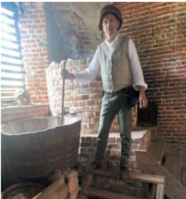
Here I'm standing by the mash tun and about to open the tap to let the hot water run in from the copper
