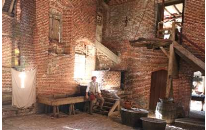
The brewery, with Dirk standing by the cooling tray. The copper is within the circular brickwork behind him, the mash tun is also just behind him, and there are two fermentation tuns on the floor
