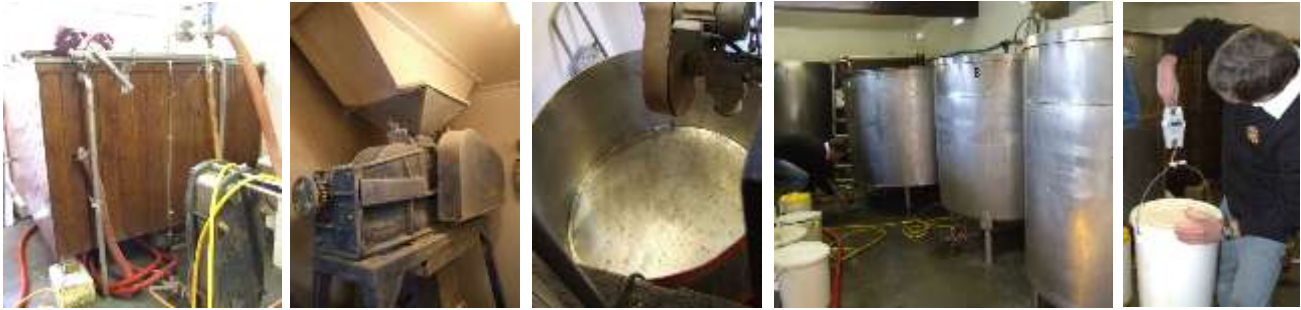
Burton Bridge hot liquor storage tank with the paraflo in the foreground; the trusty Bentall two roller mill; the mash tun with its 9000 hole false bottom; some of the fermenters and Bruce weighing out the yeast. All photos from 2008.
