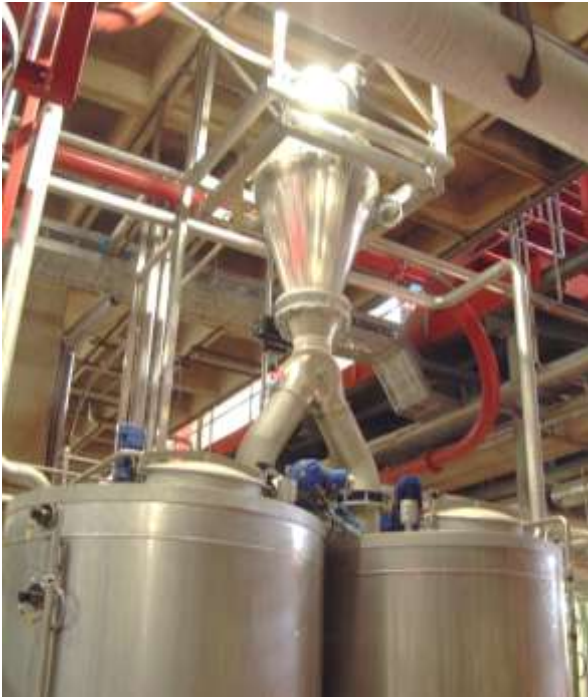
Inside Carlsberg's plant at Northampton which celebrated its 50 th anniversary in 2024. These tanks are used to slurry hop pellets before adding to the coppers.
