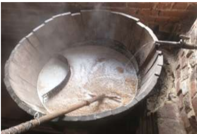
Water is running into the mash tun. There is a capstaff (wooden plug) in the bottom of the tun, which is protected by the curved basket work. At the end of the mash we withdraw the plug to run the wort into the cooling tray. On the right is one of the bakers with a jug full of yeast that he has skimmed from our fermentation tun (centre), he will be using it to bake a batch of common loaves.
