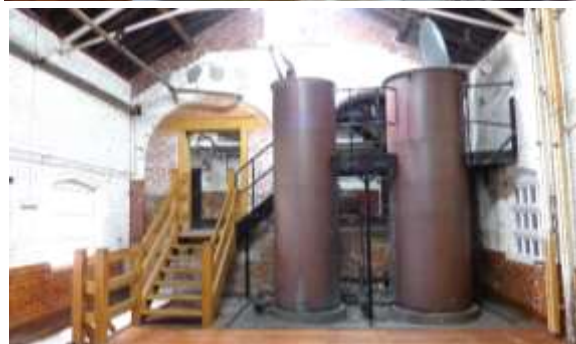
The head of the 85' deep ale liquor well; mash tun; copper and the 'dog kennels' which circulate wort from the hop backs to infuse late hop aroma.
