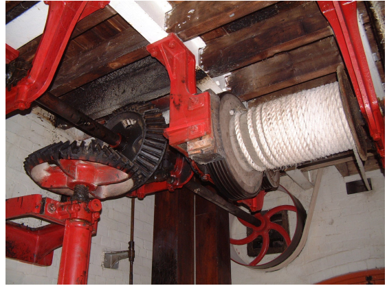
Figure 18. Sack hoist at Hook Norton.
