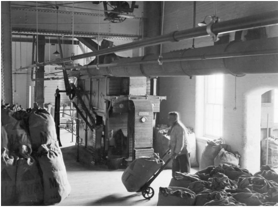
Figure 3. The malt screens in Bass' No2 Brewery, Burton (NBHT).
