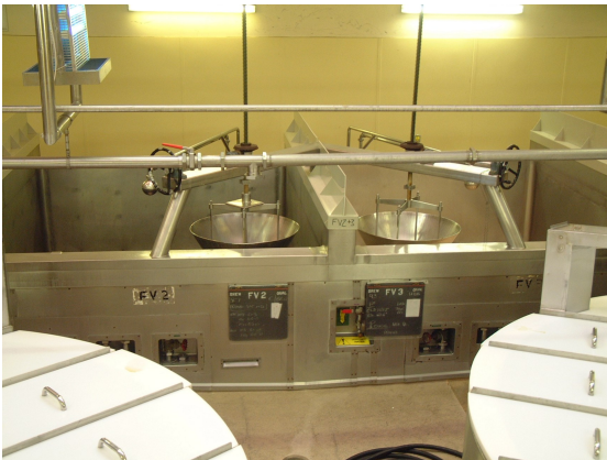
Figure 69. Open stainless vessels complete with parachutes for skimming at Robinson's.
