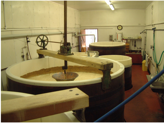
Figure 67. Lined wooden fermenters at Batham's.
