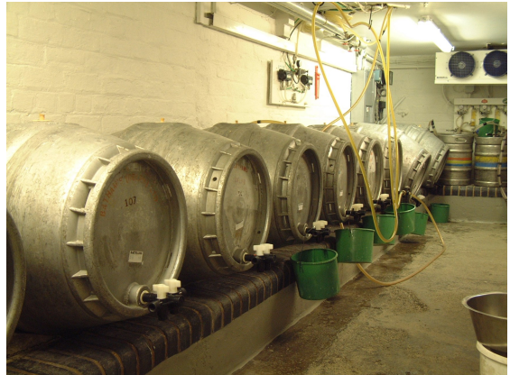
Figure 95. The cellar at the Bull and Bladder beside Batham's plant at Brierley Hill. These are epoxy lined cast aluminium barrels ...
