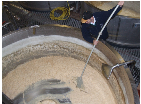
Figure 76. Skimming the yeast from the top deck of a Yorkshire vessel (Black Sheep 2006).
