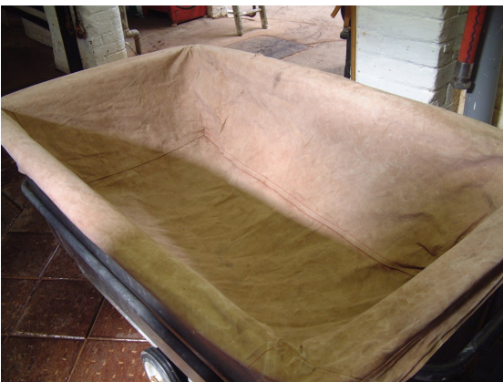
Figure 71. A yeast skip at Bathams complete with a woven cloth to allow barn ale to drip out.
