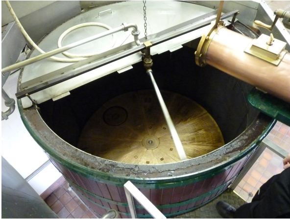
Figure 46. The mash tun at Holden's takes a charge of 375kg yielding 36 barrels a time (2012).
