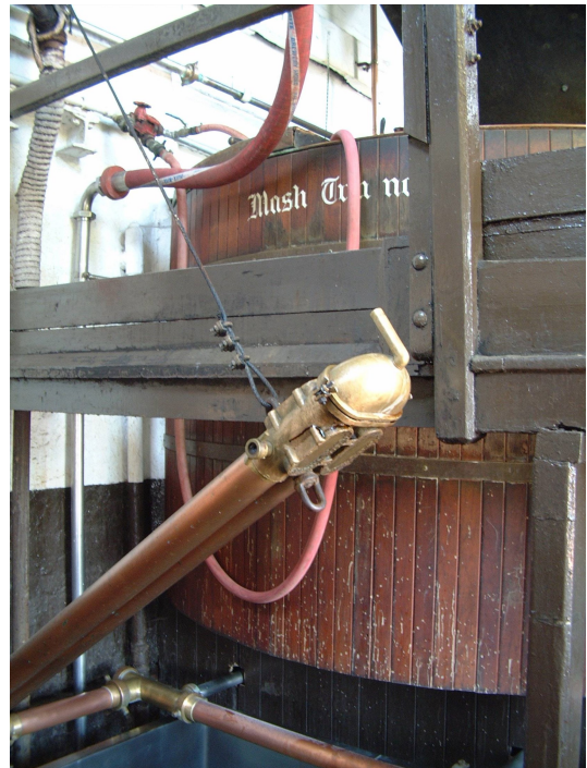
Figure 49. A Valentine swinging run off flow control device at Arkells in Swindon (2001).
