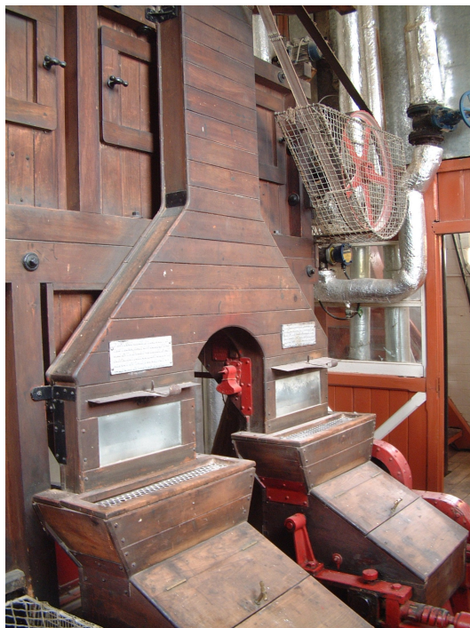
Figure 45. At Hook Norton, a screen separates large and smaller corns and they are crushed through two-roller mills with different gaps. (2002).
