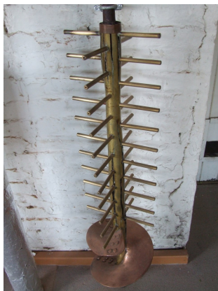
Figure 51. The innards of a Steel's masher at Elgoods in 2006. Note the screw to move grist forward and the tines to mix the water in.
