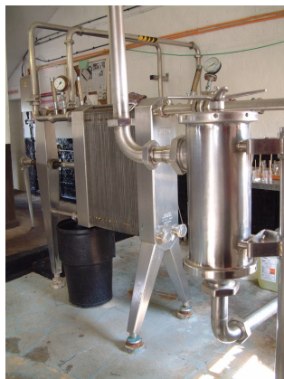
Figure 62. The more hygienic stainless steel paraflow at Arkells. Note the hop seed filter in the foreground (2001).
