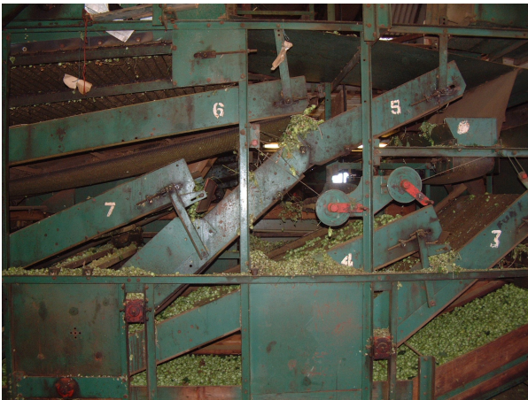
Figure 34. Hop picking machine at Claston Farm.
