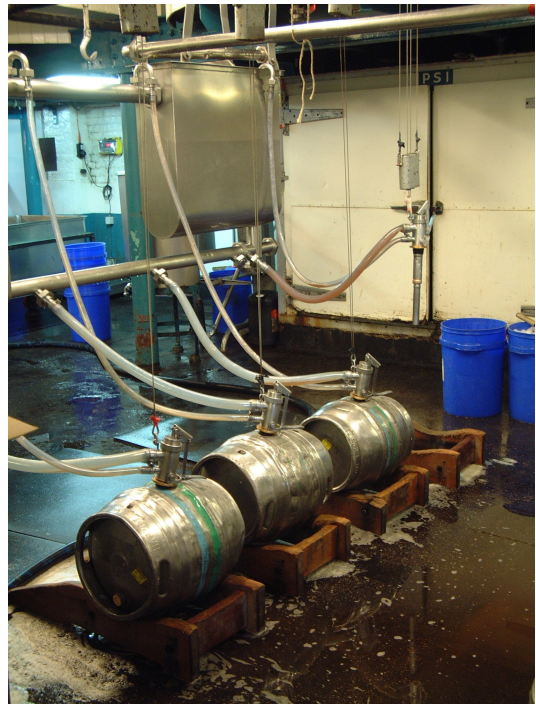
Figure 98. Filling metal casks at Harveys (2004).
