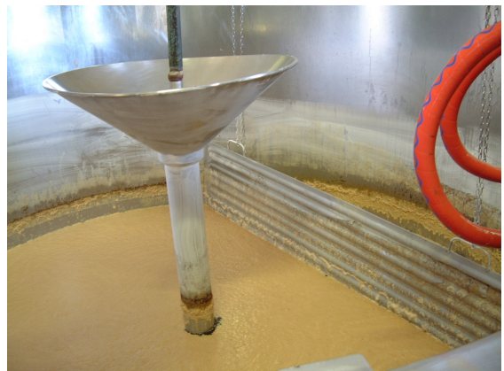
Figure 72. A parachute at Harveys wound back up after use. Note the attenuation panel.
