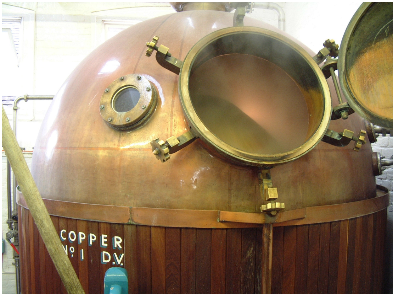
Figure 38. This 60bbl copper at Harveys in 2004 was built by Scottish coppersmiths Forsyth in 1999.
