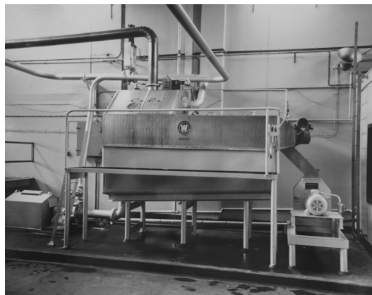
Figure 43. The Wittemann hop separator at Castlemaine Perkins in Brisbane.
