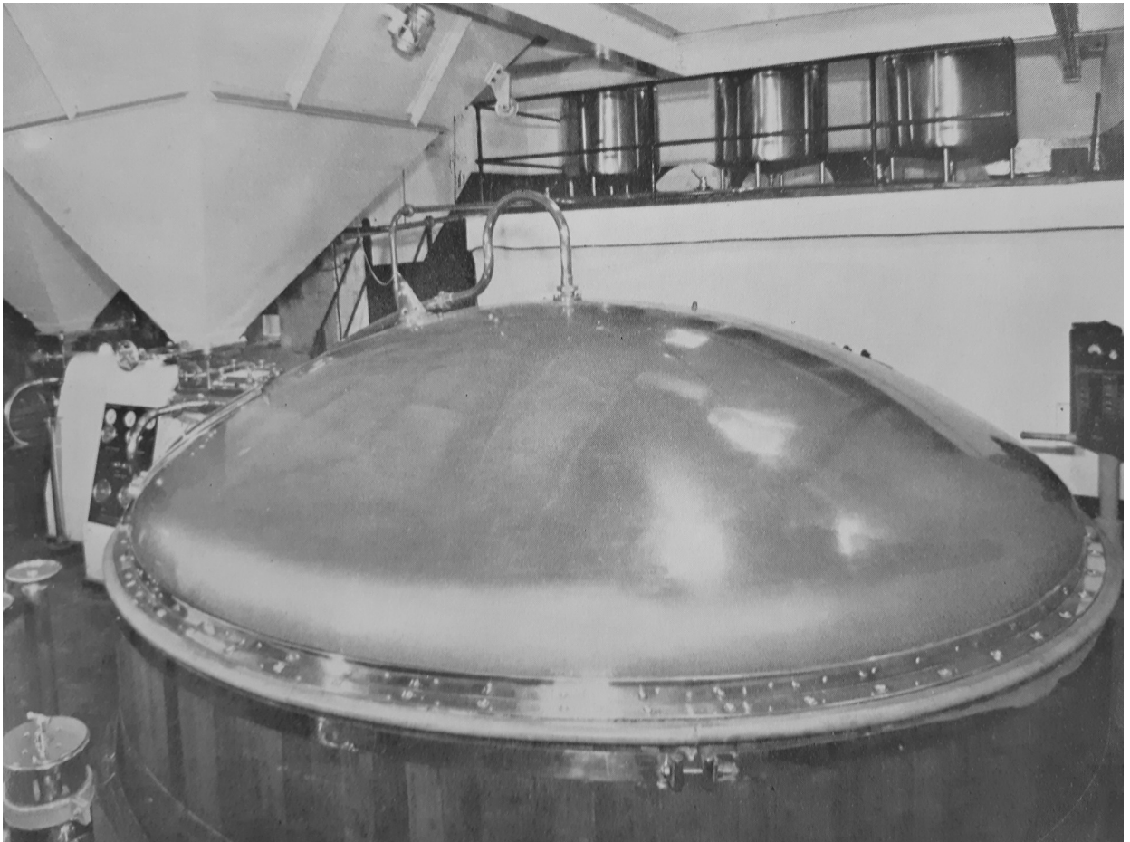
Figure 4. Mash tun, showing mixer above tun.
