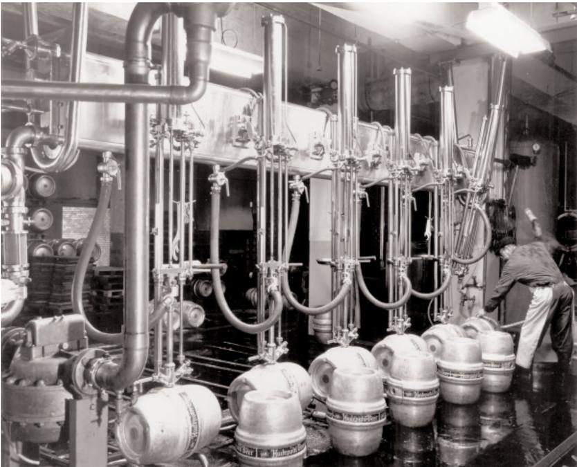
*Figure 16. Filling and sealing quarter-barrel kegs in the old Hudepohl racking room, circa late 1970s. (Hudepohl-Schoenling Brewing Company archives)*
