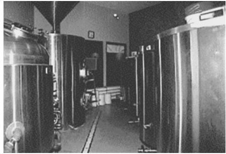
Figure 2. Seven stainless steel fermenters are open and glycol jacketed with a total capacity of 80 hectoliters at the Flat Branch brewery.
