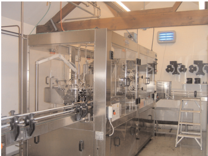
Figure 8. The eight head filler with change parts hung on the wall.
