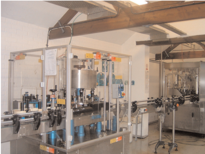
Figure 7. In the bottling hall - The labeler with filler in the background.
