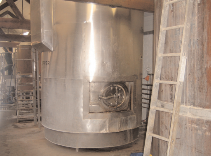
Figure 6. The gas-powered 30 barrel kettle.
