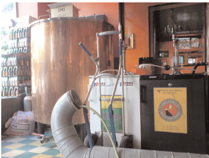
Figure 3. On the left, the fermenting tank with a volume of approximately 1,300 litres. On the right, a 20 litres keg fridge for private events and, above, a window with a view onto the brewery from inside the pub.
