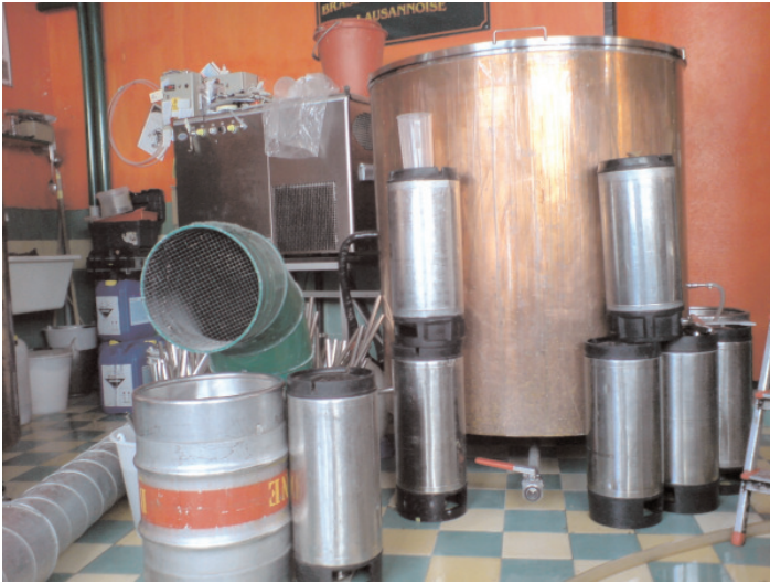
Figure 4. On the left, the cooling system and on the right a fermenting tank also approximately 1,300 litres in capacity.
