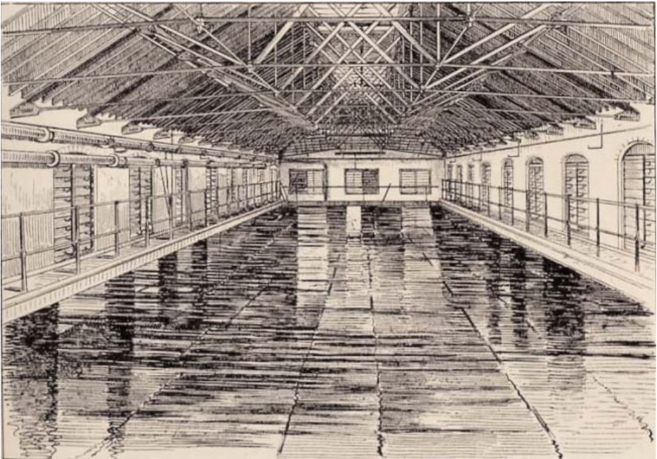
Figure 4. An open cooler at John Smith's brewery, Tadcaster, from Alfred Bernard's Noted Breweries of Great Britain and Ireland, volume 3, published in 1890.
