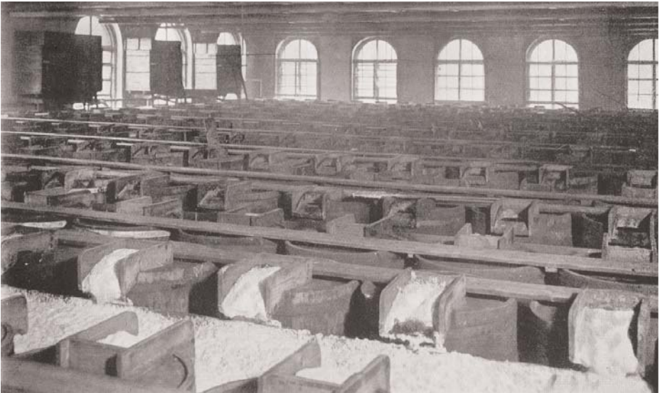
Figure 9. The Ponto system of fermentation in operation in an unnamed brewery, from Julian L. Baker's The Brewing Industry, published in 1905.
