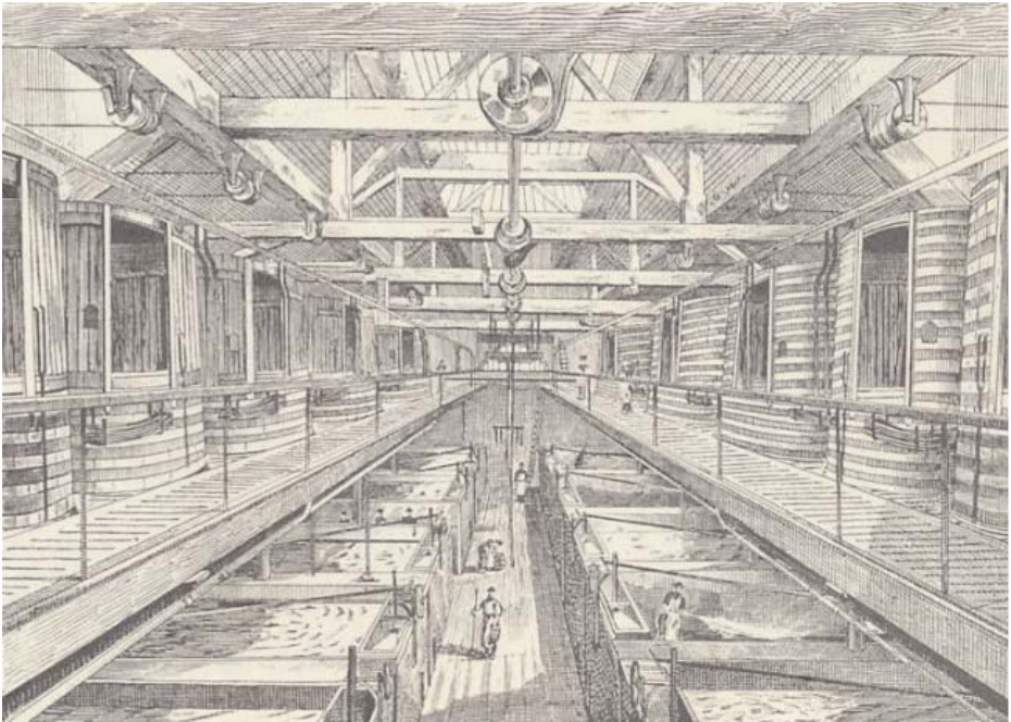
Figure 7. The dropping system of fermentation in operation at Jacob's Street brewery, Bristol, from Alfred Bernard's Noted Breweries of Great Britain and Ireland, volume 2, published in 1889.
