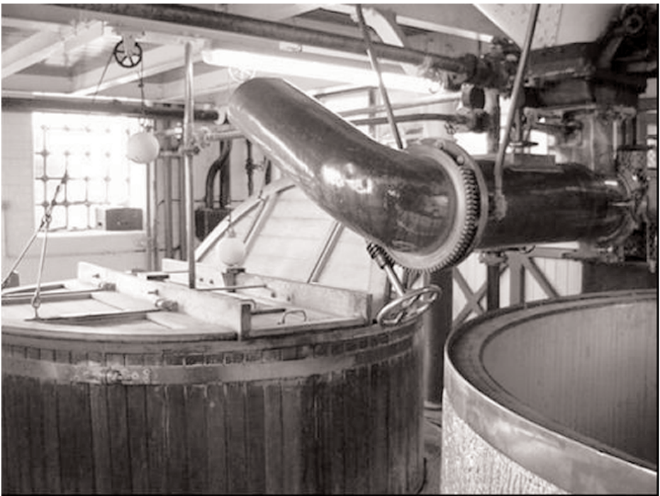
Figure 3. A Steel's Masher at Hook Norton brewery. Photograph courtesy of Roger Putman 2004.
