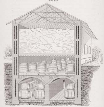
Figure 13. Lager fermentation and maturation in an ice-house, consisting of an underground store-cellar with a fermenting cellar above it, both cooled by the natural ice in the upper part of the building, from Julius E. Thausing's, The theory and practice of the preparation of malt and the fabrication of beer, published in 1882.
