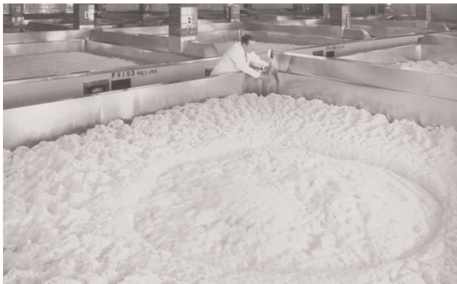
Figure 10. The Yorkshire square system of fermentation in operation at Joshua Tetley & Sons brewery, Leeds in the 1970s. Photograph from the author's collection.
